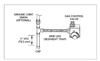
FIGURE 19. GAS PIPING WITH FLEXIBLE CONNECTOR.
